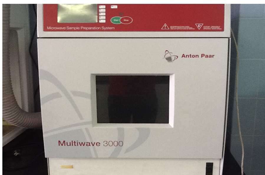
Figura 5.2- Micro-ondas Multiwave 300 Anton Paar
