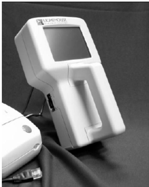
**Figura 15 – Medidor de poeiras HANDHELD 3016 IAQ Particle Counter (William,2007)**
