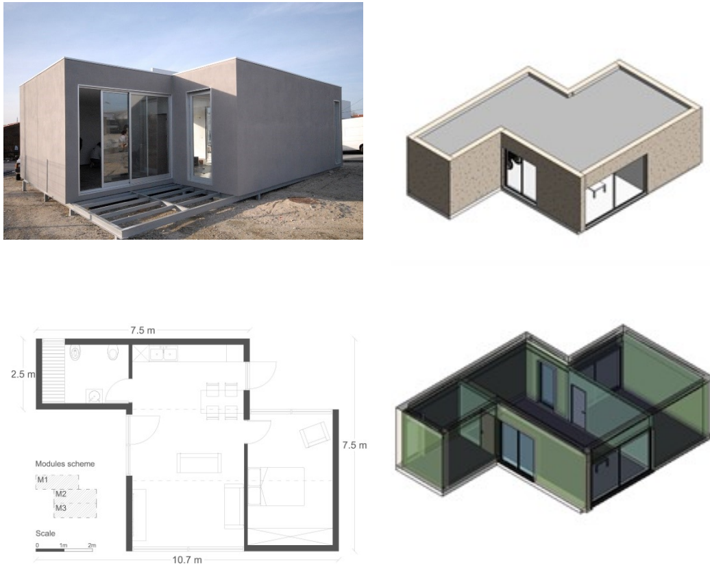
Figure 14 Prefabricated house picture and axonometric view of the BIM model, floorplan, and axonometric view of the energy model.
