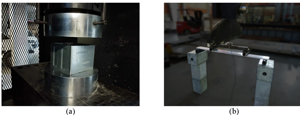
Fig. 8. Laboratory tests of the steel structural components: (a) block and (b) deck board.
