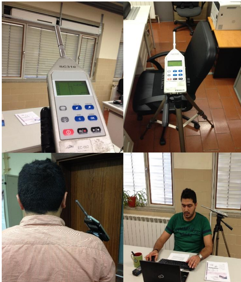
Figure D. 2 – Noise measurement device and setup.
