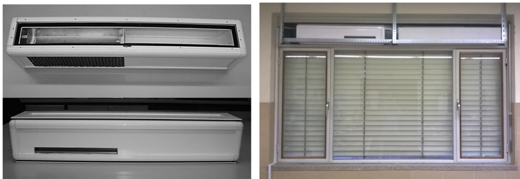
Fig. 10. Prototype of the mechanical ventilation subsystem of the Smart Window hybrid ventilation system.
