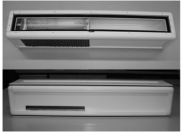
Fig. 1. Prototype of the mechanical ventilation subsystem of the Smart Window hybrid ventilation system (tangential blower).
