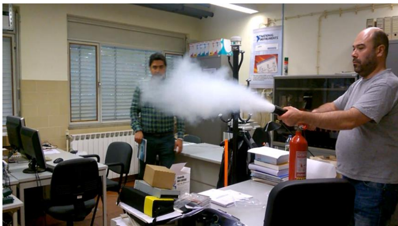
Figure 4.6 – Releasing CO 2 into the I2L office for evaluation of the AER associated to the ventilation strategies for Smart Window system.
