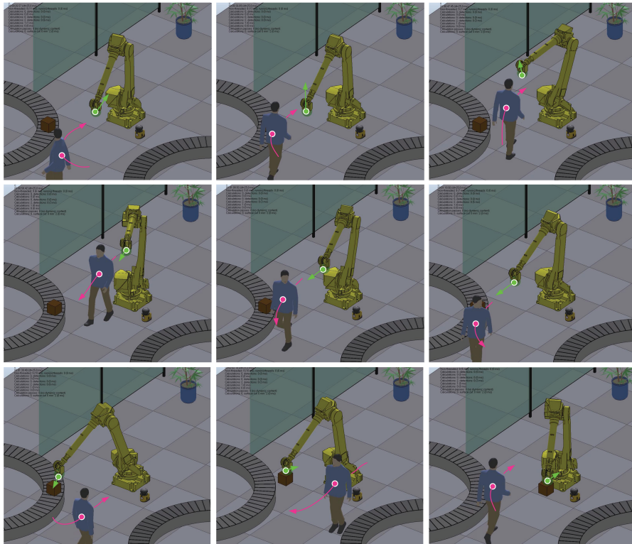
Figure 5 Demonstrates a sequence of photos of a VREP simulation for safe robotic cell, minimum distance calculation was performed using the proposed method.
