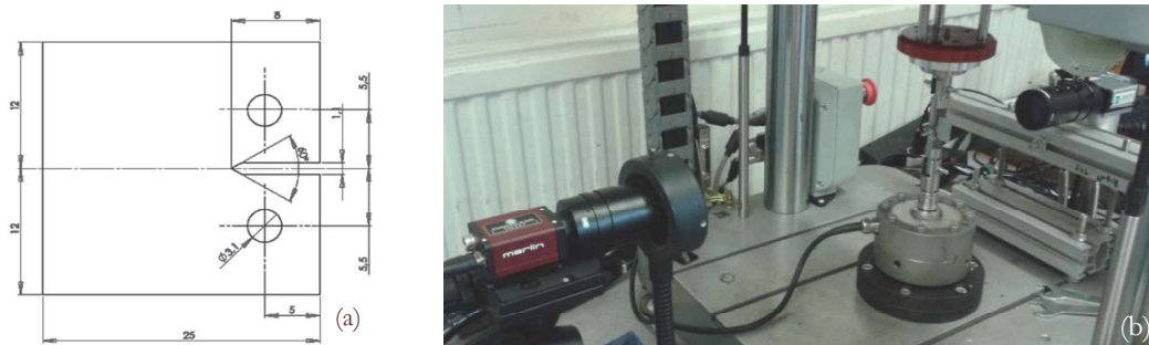
Figure 1: (a) Dimensions (mm) of the CT specimen tested. (b) Experimental set-up used to measure DIC data during fatigue testing.
