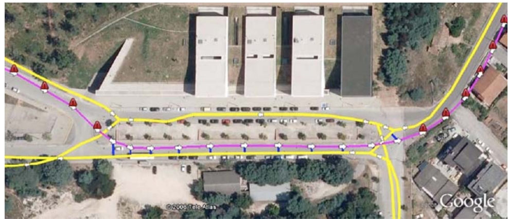
Fig. 4 Matching a new trace. Yellow lines represent the existent map and arrows represent its direction. The magenta line is the new trace. Blue lines represent the matched trace points and the triangular signs the unmatched ones
