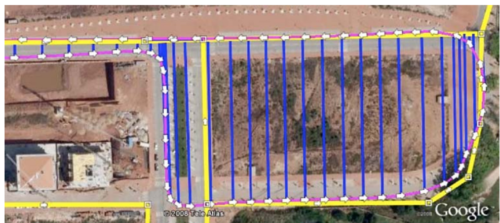
Fig. 11 Marchal's original algorithm: given the absence of a descending road in the center, the algorithm insists on keeping the match to the upper road. We recall that, in Yellow, we have the "base map"; in magenta, with arrows for direction, we have the incoming trace; in blue, we have the matches connecting the trace to the base map
