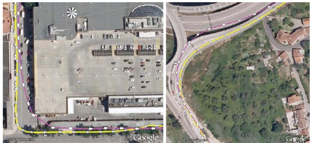
Figs. 5 – 6 Difference between map and trace patterns in curves. The yellow line represents the map and magenta the trace
