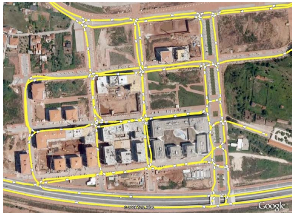
Fig. 24 Map generated from scratch out of 24 traces (2,926 points)
