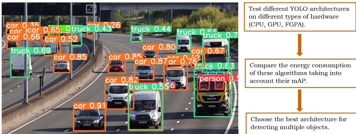
Figure 1.1: Example of YOLOv5s network detection output for an image (left). Diagram of the steps performed (right).
