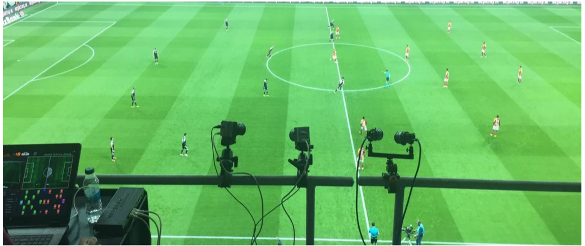
Figure 1. Sentio Sports optical tracking system positioning.
