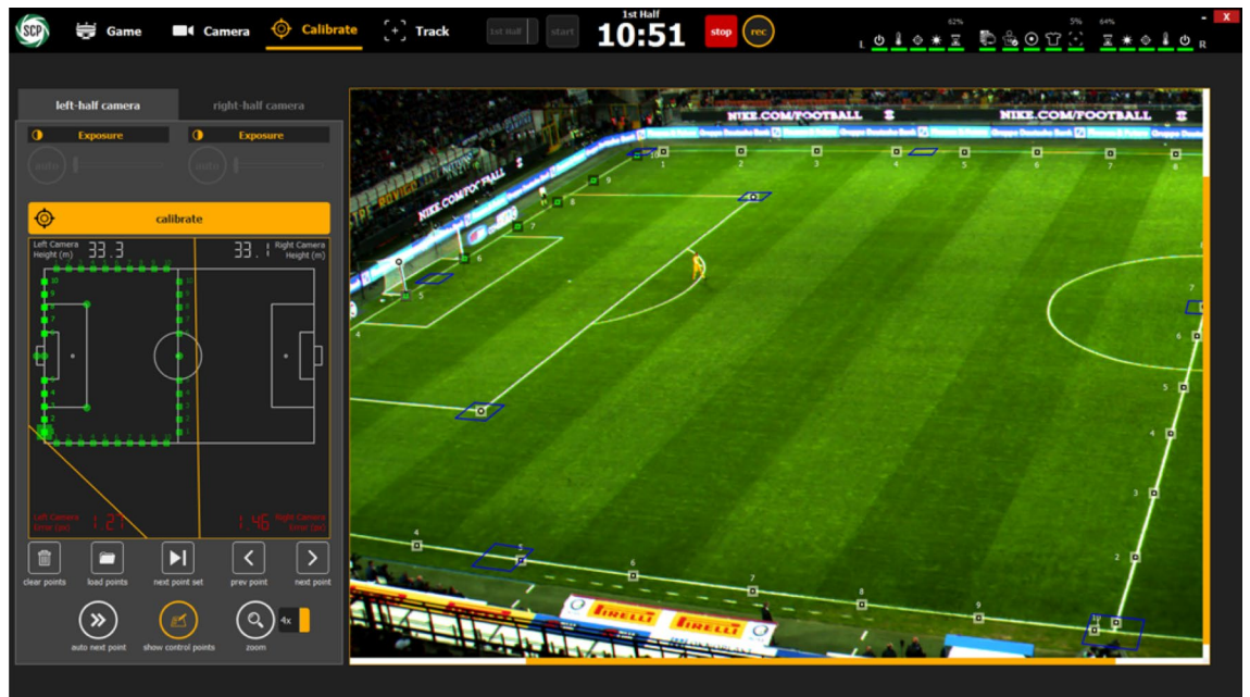
Figure 3. Sento Sports optical tracking system field calibration.
