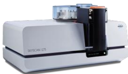
Figure 28. Micro-CT (X-ray microcomputed tomography) equipment.
