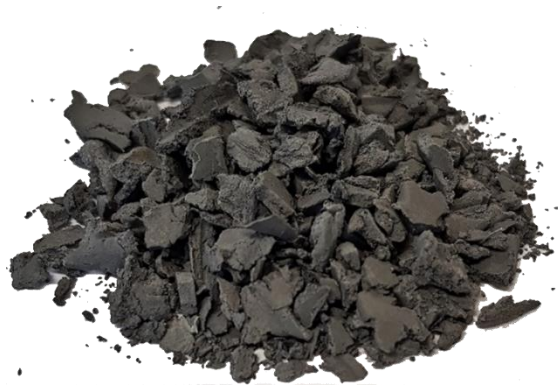
Figure 36. Pellets of NiTi feedstock.
