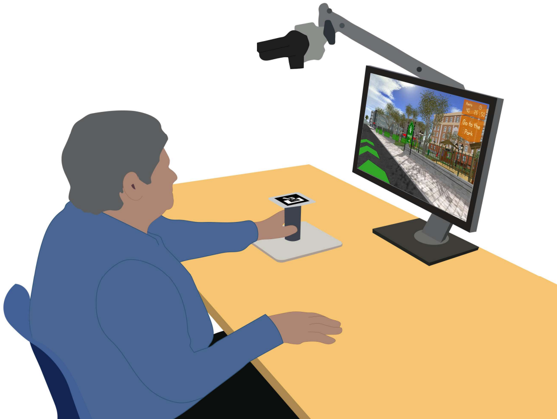
Figure 5: Reh@City v2.0 experimental setup. The user faces an LCD monitor and moves a handle on the surface of the table with his/her paretic arm to interact with the virtual content.
