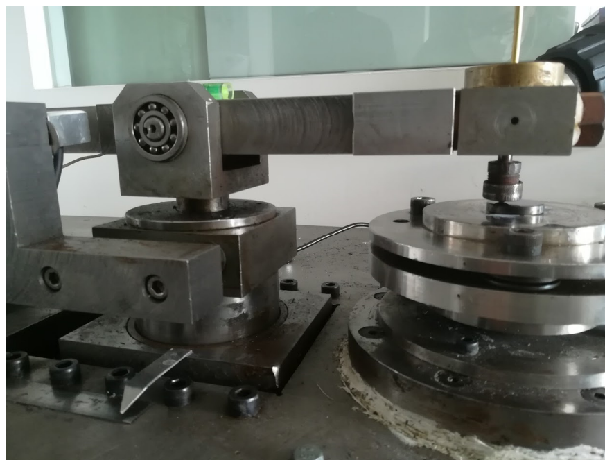
Figure 1. Customized pin-on-disk (POD) machine utilized for tribological testing.
