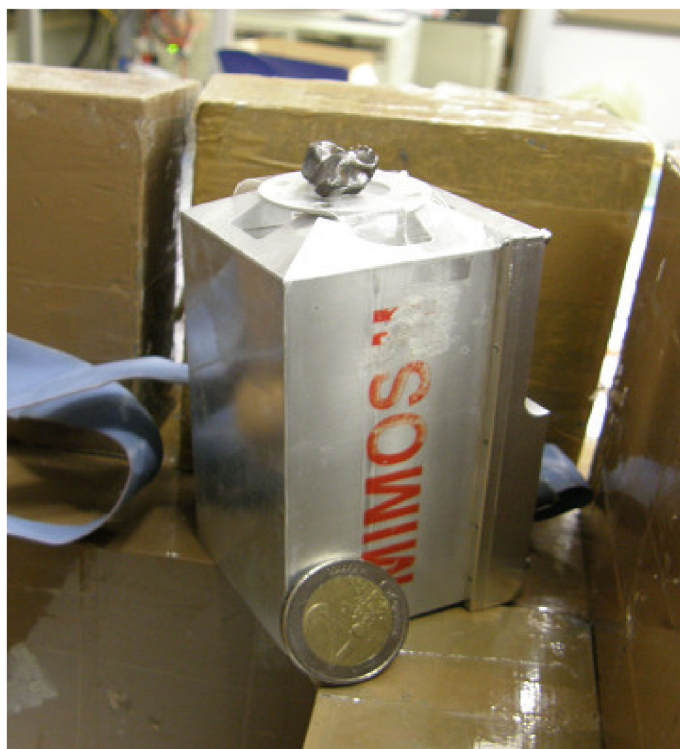
Figure 6. MIMOS II spectrometer measuring an iron meteorite placed on top of the window.
