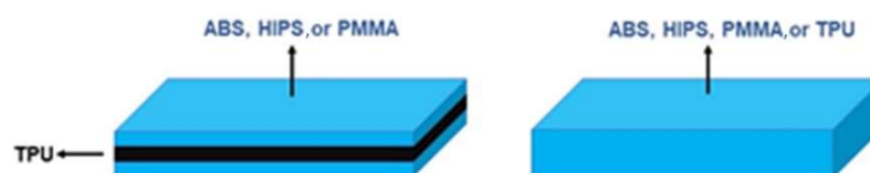
Figure 1. Schematic representation of the printed sandwich structures with ABS, HIPS, or PMMA as skins, and TPU as the core material (left) and mono-material specimens (right).
