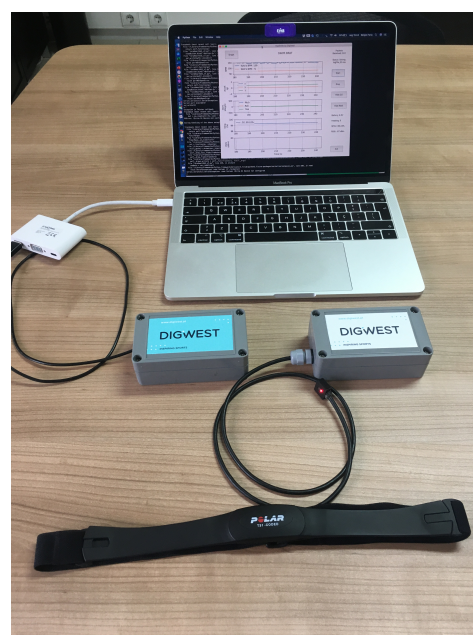
Figure 2. Hardware setup: the wearable device (on the right—white label) and the base station module (on the left—blue label).
