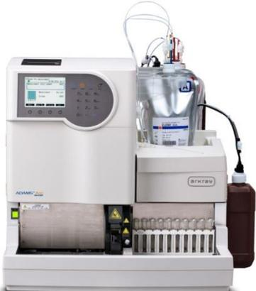
An ADAMS A1c HA-8180V hemoglobin A1c analyzer, a white laboratory instrument with a sample tray and a small display, used for automated HbA1c measurement.              |
