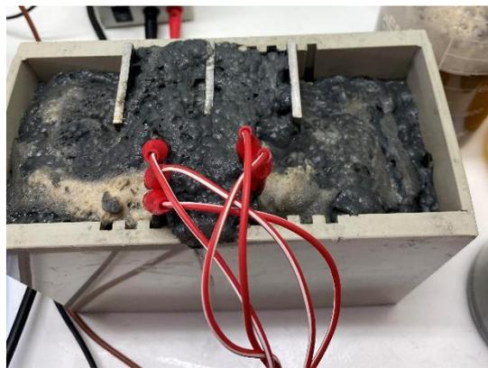
**Figura 5.13** - Espuma formada na amostra AL5 ( $J= 15 \text{ mA/cm}^2$ ,  $NE=5$ ,  $t=30\text{min}$ ).
