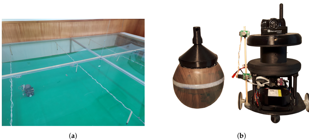
Figure 4. Experimental setup. (a) Wind tunnel environment; (b) odour source (left) and mobile robot (right).
