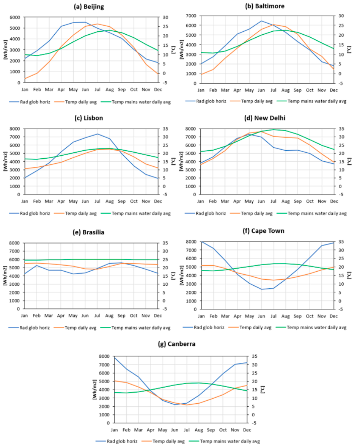
Figure A1. Evolutions of the average global horizontal solar radiation, the average daily ambient temperature, and the average daily mains water temperature throughout the year at the seven assessed locations: (a) Beijing; (b) Baltimore; (c) Lisbon; (d) New Delhi; (e) Brasília; (f) Cape Town; (g) Canberra.
