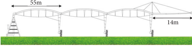
FIGURE 3: Structure of the pivot used in the presented case study.
