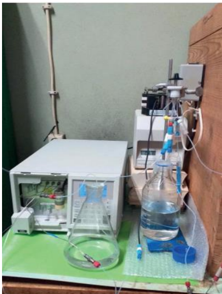
Figure 6. Equipment used in Taylor Dispersion Technique.
