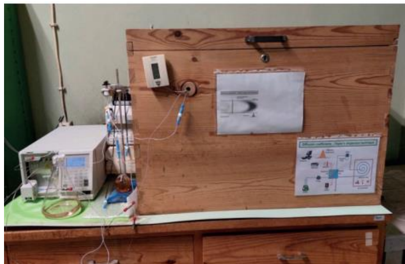
Figure 6. Equipment used in Taylor Dispersion Technique.
