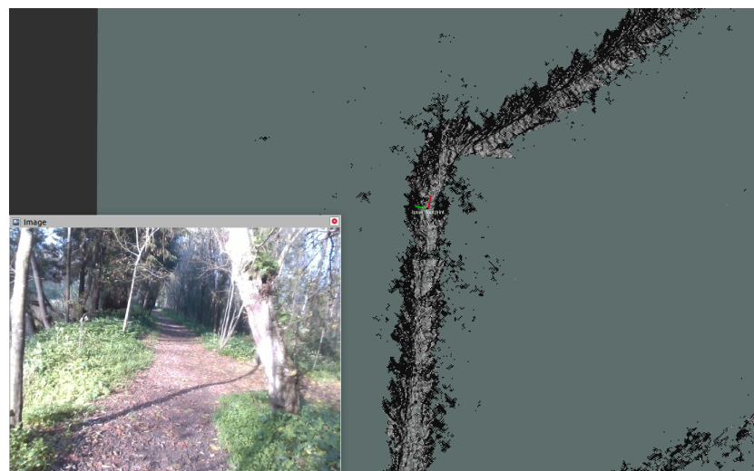
Figure 12. Mechanical effort costmap generated by the method presented in [54] with data from our dataset, in which lighter values in the grayscale represent easier to traverse areas and vice versa.
