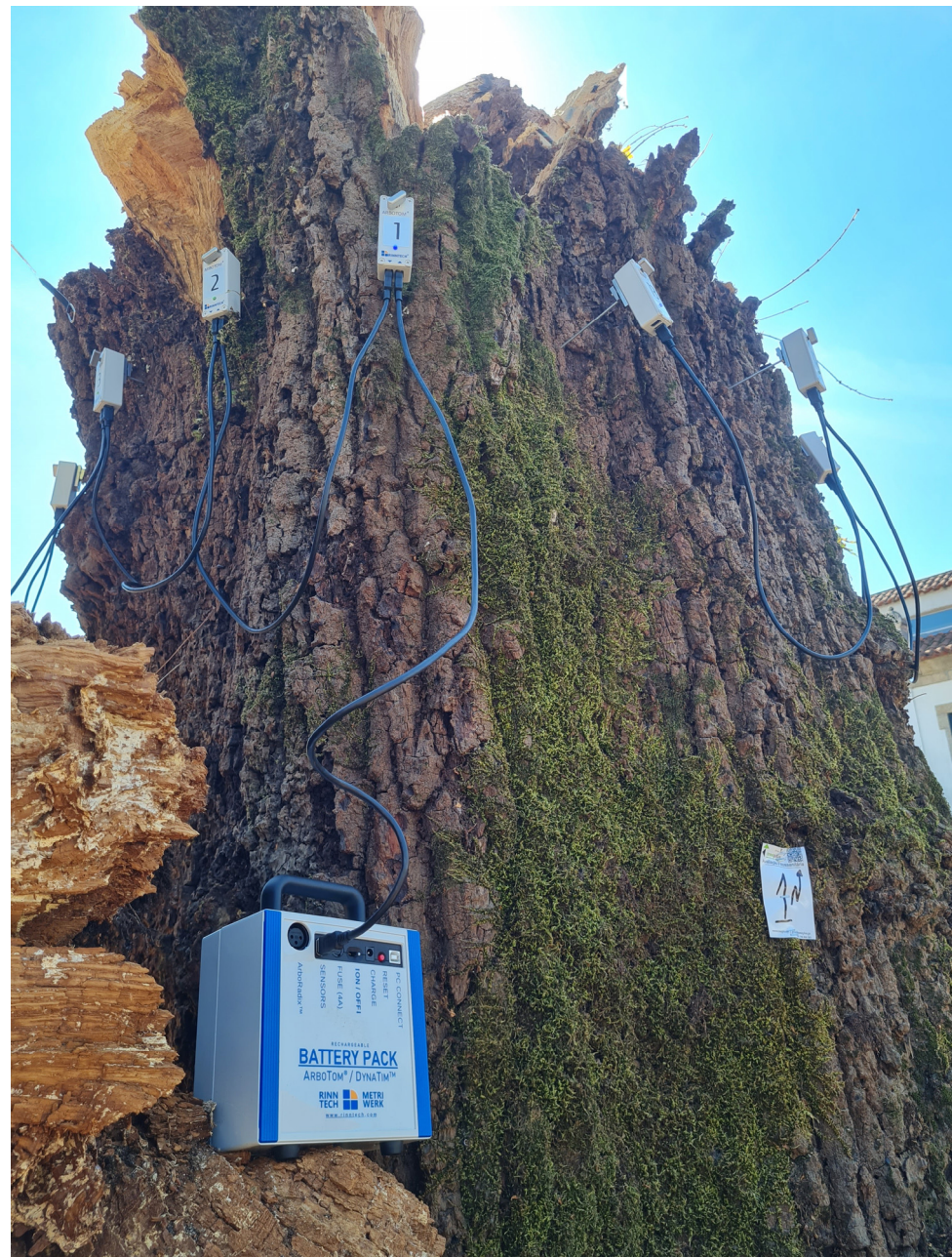
Figure 3. Example of the distribution of the Arbotom sensors on the stem of an oak tree.
