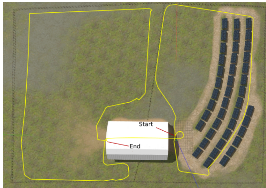
Figure 5. Ground truth trajectory of the robot (depicted in yellow) in the simulated agriculture environment.
