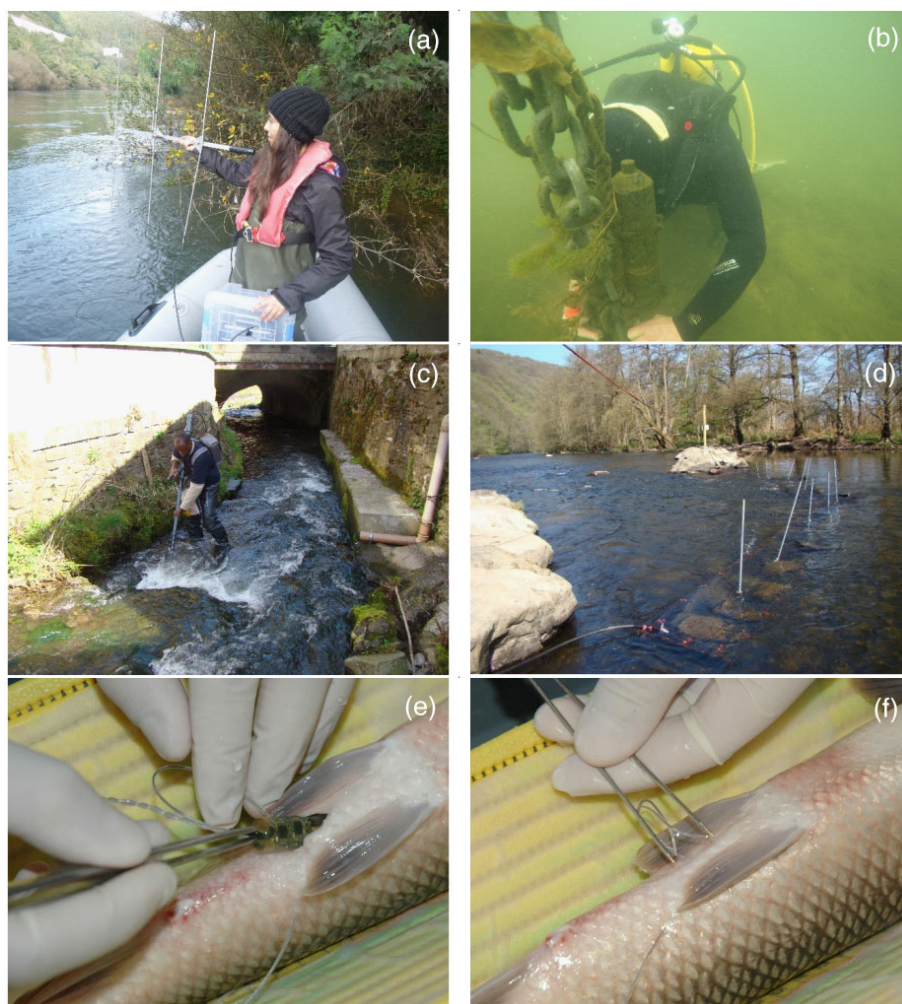
FIGURE 1 Biotelemetry techniques used to study fish movements in rivers: (a) manual tracking with radio telemetry receiver and hand held Yaggi antennae (photo by Carlos Alexandre); (b) passive tracking with acoustic telemetry receiver (photo by Bernardo Quintella); (c) manual tracking with a portable passive integrated transponder (PIT) antenna (photo by University of Liège-LDPH); (d) instream submersible stationary PIT antenna (photo by University of Liège-LDPH); (e) surgical implantation of an electromyogram (EMG) radio transmitter on an Iberian barbel Lucioibarbus bocagei (photo by Carlos Alexandre); (f) detail of the gold electrodes of the EMG transmitter that will be secured on the red axial musculature to detect swimming activity (photo by Carlos Alexandre) [Color figure can be viewed at wileyonlinelibrary.com ]
