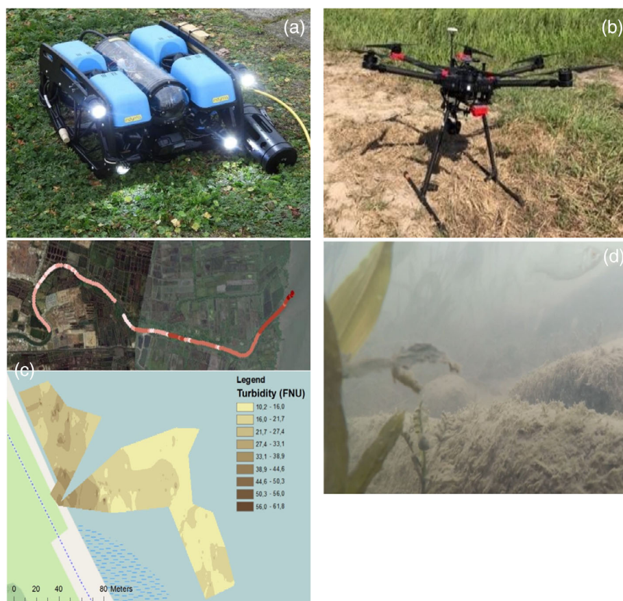
FIGURE 3 Examples of different unmanned vehicles/systems and results from data collection campaigns: (a) unmanned underwater vehicles equipped with cameras and water quality sensors; (b) unmanned aerial system, including multirotor drone equipped with sensors; (c) water quality mapping using aquatic drones equipped with sensors: electrical conductivity (top) and turbidity (bottom) in different sections of rivers (datasets obtained during a climate café workshop); (d) snapshot of underwater environment (fish, sediments and vegetation) captured with an aquatic drone at the river Maas, in The Netherlands (all photos by Rui Lima) [Color figure can be viewed at wileyonlinelibrary.com ]
