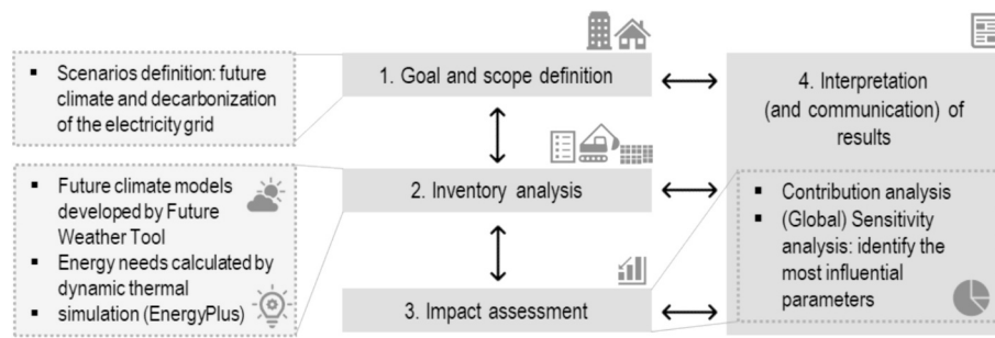
Fig. 1. Prospective life cycle methodological approach framework for building retrofits' adaptation for future climate scenarios. Adaptation from the life cycle assessment framework recommended by ISO 14040/14044 [21,22].
