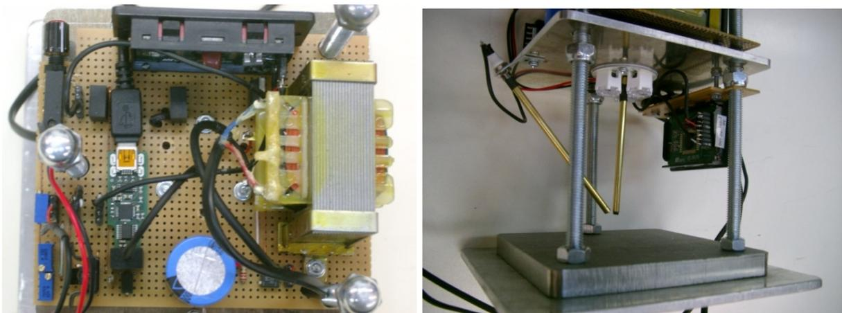
Figure 9– Different views of the experimental setup A: on the left, a top view, and on the right, a lateral view showing the different light sources.
