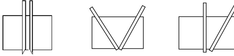
Figure 15 – The different measuring heads used in Experimental setup D. On the left, a measuring head with a configuration of  $0^\circ/0^\circ$ ; in the middle, a configuration of  $45^\circ/45^\circ$ ; on the right, a configuration of  $45^\circ/0^\circ$ .
