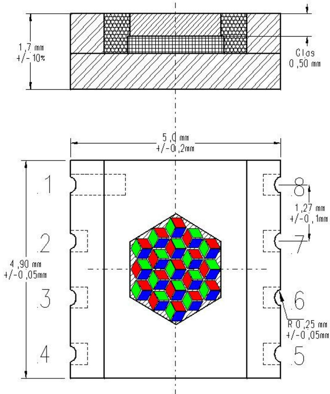
MTCSiCS in 8 Pin LCC package (side view and front side)
