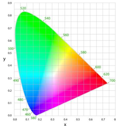
Figure 5– The CIE 1931 colour space chromaticity diagram (12).
