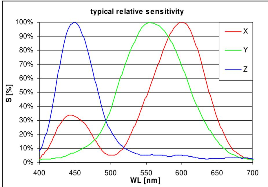
Figure: Typical (relative) sensitivity (XYZ) of the color sensor (MTCSiCS) scanned by width broadband light<sup>3</sup>,
