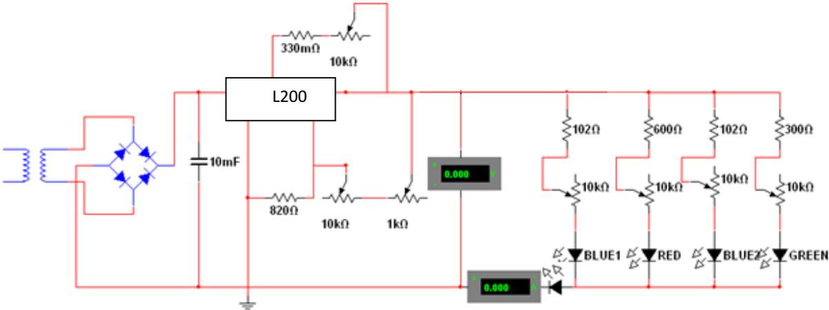
Figure 17 - Schematic diagram of the circuit used for the RGB LED in Experimental setup D.
