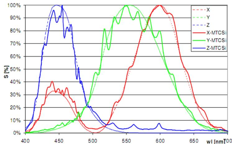
**Figure 19 - Typical (relative) sensitivity (XYZ) of the colour sensor (MTCSiCS), and Standard Observer function (34).**
