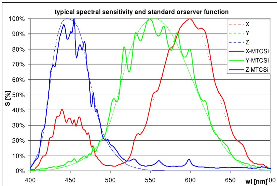
Figure: Typical (relative) sensitivity (XYZ) of the color sensor (MTCSiCS), scanned by narrow-band light<sup>4</sup>
