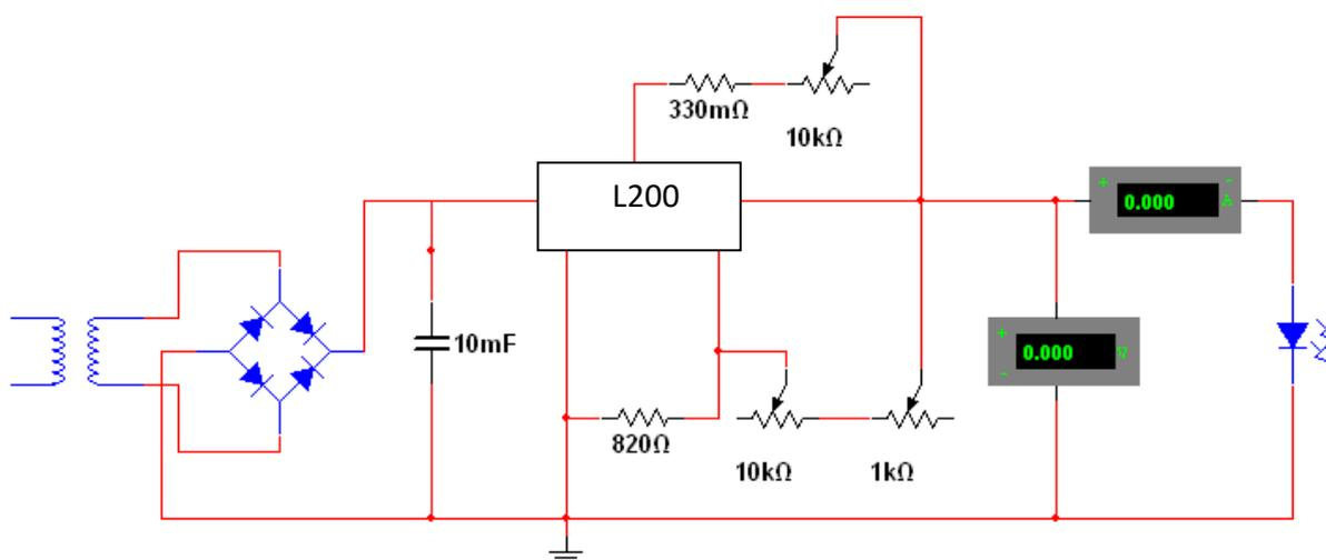
Figure 10 – Schematic diagram of the current regulator of Experimental setup A.
