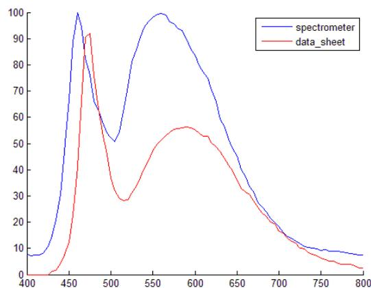
**Figure 22- The high intensity LED spectrums: one given by its data sheet, and the other given by the spectrometer.**
