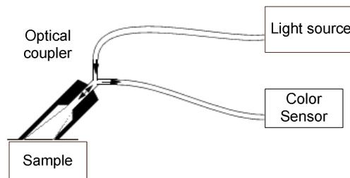
Figure 11- Schematic diagram of experimental setup B (31).
