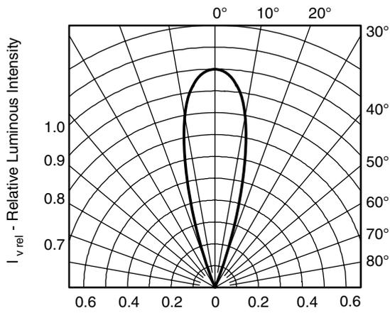
Figure 8. Rel. Luminous Intensity vs. Angular Displacement
