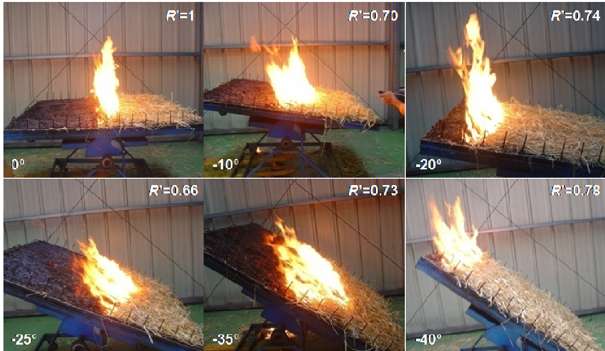
Figure 4.16 – Flame geometry and non-dimensional ROS as a function of slope for tests in the range 0^\circ \leq \alpha \leq 40^\circ . The variation of the flame geometry for different slope angles can be observed, fuel bed: straw, fuel load: 0.6 \text{ kg/m}^2 .
