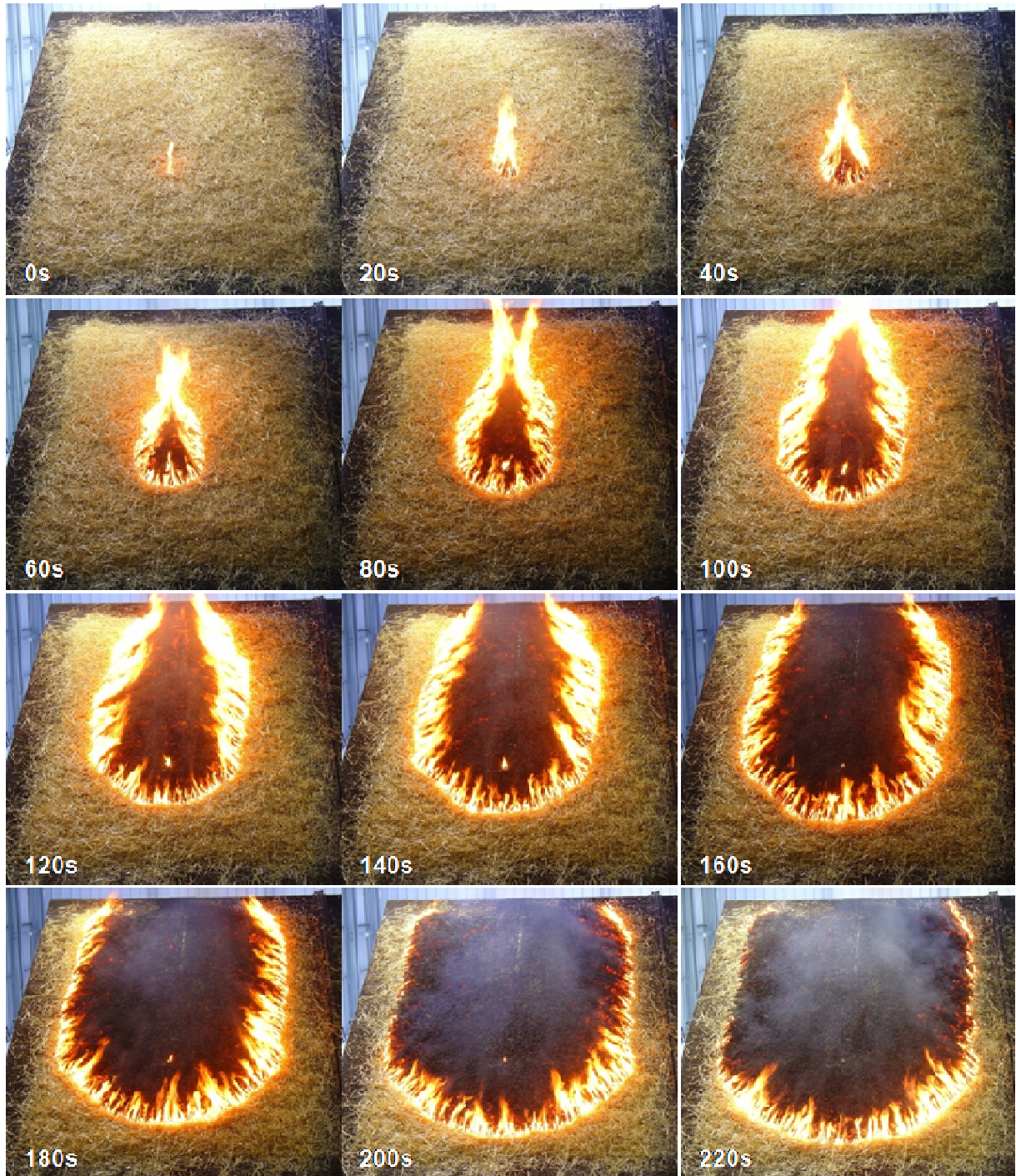
Figure 4.30 – Sequence of pictures for the experiment FL-DE4-01 on the Canyon Table DE4, fuel bed: straw, fuel load: 0.6\text{kg/m}^2 , slope: 30^\circ . The time since ignition is indicated in each picture.
