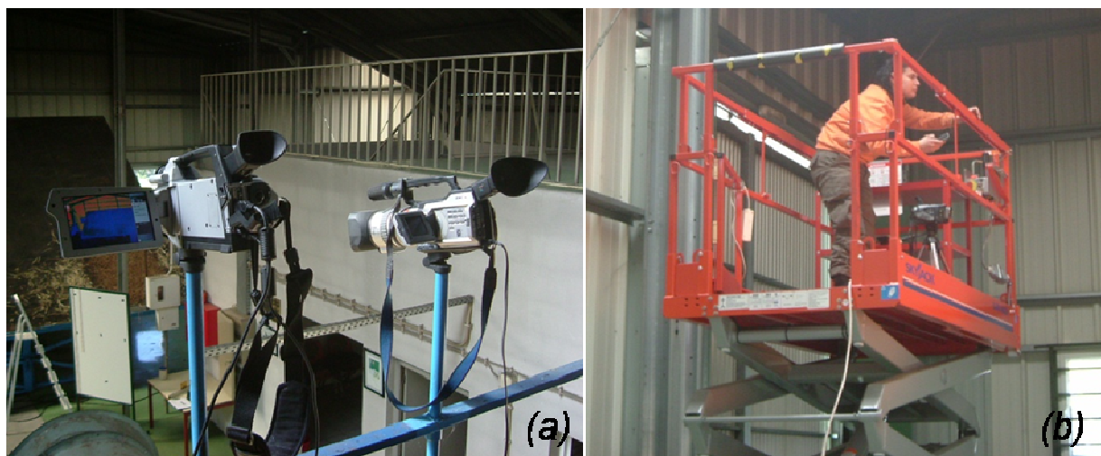
Figure 3.4 – Image recording of the DE4 test rig: (a) Infrared and video images recording from the top of the table. (b) Video images recording from the side of the table.
