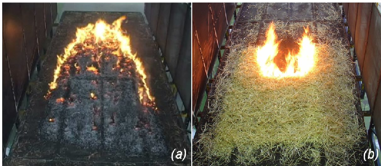
Figure 3.3 – Experiments in the Combustion Tunnel TC2, fuel load: 0.6 \text{ kg/m}^2 : (a) Ref.: FR-TC2-07, wind velocity: 2 \text{ m/s} , fuel bed: pine needles. (b) Ref.: BR-TC2-04, wind velocity: -2 \text{ m/s} , fuel bed: straw.
