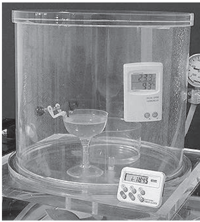
Figure 4: On the left: setup for our experiments on the humidity dependence of the drinking bird period. The bird is placed inside a closed transparent chamber. A digital chronometer and a digital hygrometer complete the set. The humidity, which started around 50%, was increasing during an experiment. On the right: logarithm of the period, \ln \tau , versus \ln(100 - H) . Two different evaporation regimes are observed, one for high (black circles) and the other for low (black squares) humidities. The changing from one regime to the other occurs at \ln(100 - H) = 3.2 . Least squares fits yield \ln \tau = 9.44 - 1.82 \ln(100 - H) for low humidities and \ln \tau = 7.69 - 1.24 \ln(100 - H) for high humidities. The open circles are the results of the simulation presented in Sec. 4.
