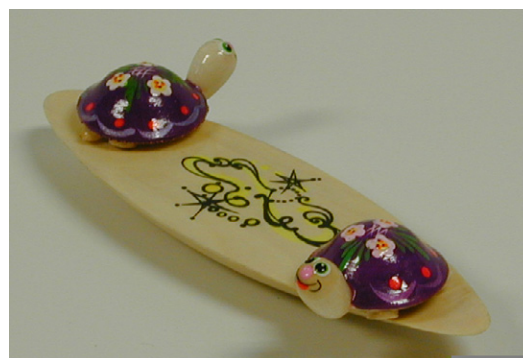
Figure 5. A wooden model of a rattleback. When rotating clockwise it rotates like any other rotating object. When rotating counterclockwise, i.e. in the opposite direction to the turtles, it eventually stops, rattles and begins to rotate backwards.
