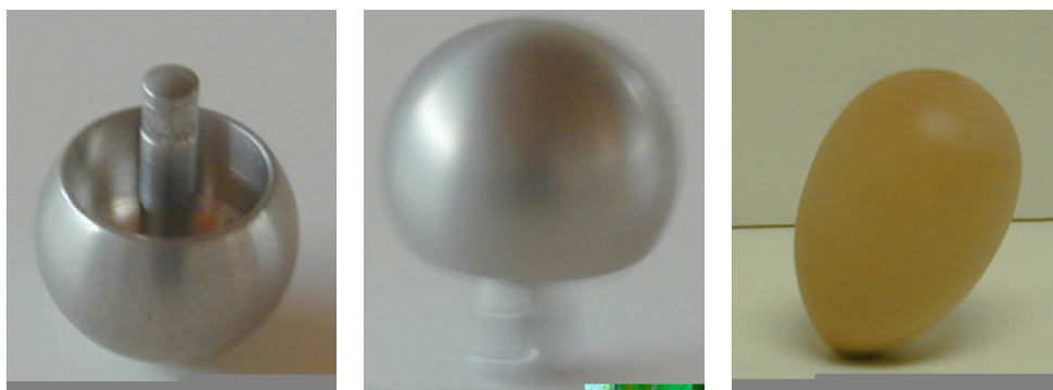
Figure 4. A tippe top is a section of a sphere with a rod (left). After spinning on its rounded body it flips over and continues rotating around its elongated stem (middle). The same happens with a rotating wooden egg (right).
