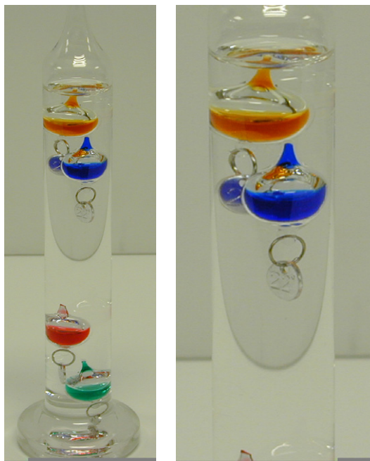
Figure 11. Galileo's thermometer. The balls inside a liquid, containing a coloured fluid, sink or float according to the value of the room temperature: they are a kind of Cartesian diver. The temperature is indicated by the lowest ball which still floats.
