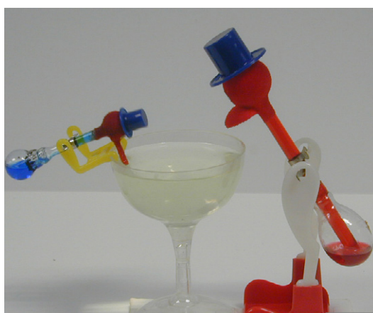
Figure 16. Two drinking birds. The water in the bird's head evaporates, the internal liquid rises, the bird inclines and 'drinks', the liquid returns afterwards to the body, and another cycle starts. The smaller bird 'drinks' more quickly.
