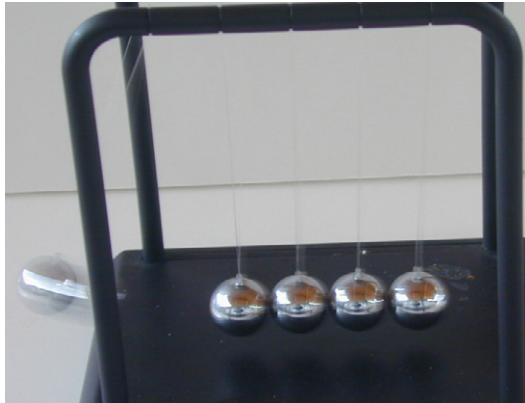
Figure 6. Newton's cradle, which follows the original Gravesande design for studying collisions. One or more balls at one side collide with the intermediate balls, causing the same number of balls to rise at the other side.
