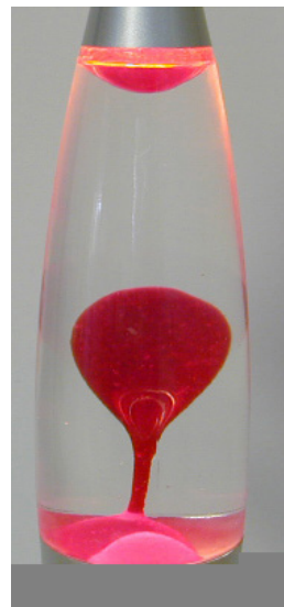
Figure 12. Lava lamp. Thermal expansion, Archimedes buoyancy, and surface tension are responsible for the amazing dynamical processes observed.
