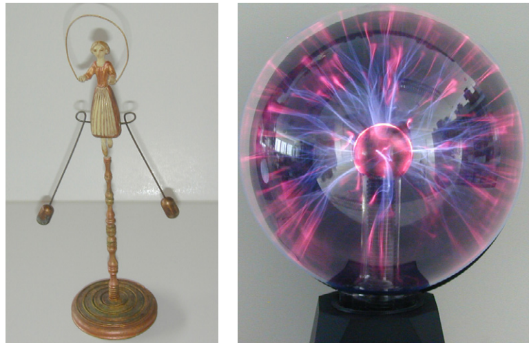
Figure 1. The old balancing toy (left) does not fall down, since a torque always acts towards equilibrium. In the modern plasma ball (right), electrons emitted by a metallic surface at the centre collide randomly with excited atoms of a gas at low pressure.
