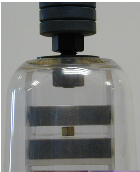
Figure 20. Levitating magnet (cube) in between two diamagnetic graphite plates and with ferrite magnets at the top. The unstable equilibrium between the magnetic force (up) and gravitation (down) is stabilized by the diamagnetic material.
