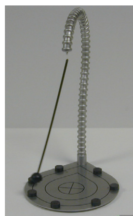
Figure 19. Chaotic magnetic pendulum: the ball, subject to a non-harmonic potential, performs a deterministic chaotic motion, i.e., a motion very sensitive to the initial conditions, although ruled by simple laws.
