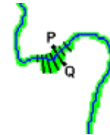
Figure 3 – Lines perpendicular to \mathcal{F} are used to determine corresponding points (P, Q) on contours \mathcal{A} and \mathcal{B} .
