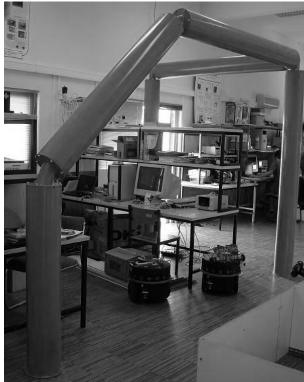
Figure 2.2: Developed structure for pole climbing robot benchmarking.
