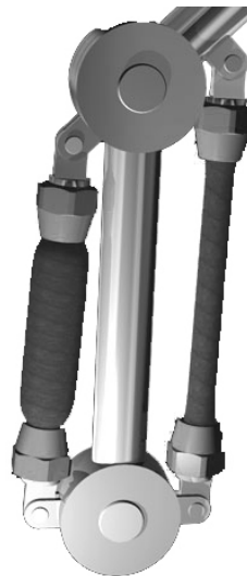
Figure 9.10: A rotational joint derived by two PMs as extensor and flexor.
