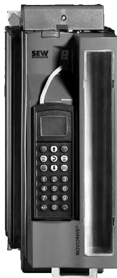
Figure A.11: MDX 60/61B driver from SEW is used for control of AC motors of the 3-DOF serial arm
