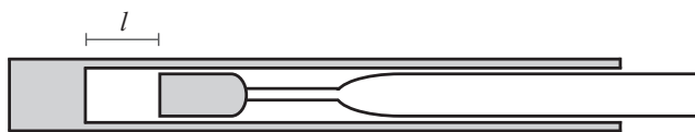
Figure 2.8: Schematic diagram of a susceptibility matched NMR tube. The sample is contained in a cylinder of length l . The bottom of the tube and the glass plug at the top of the sample have their magnetic susceptibility approximately matched to the solvent used.
