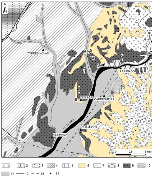
Fig. 3. Geological map of the study area and adjacent Tejo valley (adapted from 1/50,000 geological maps). 1: gneisses and other metamorphic rocks; 2: granites; 3: Jurassic (mainly limestones); 4: Cretaceous (sandstones, marls and limestones); 5: Palaeogene (conglomerates, sandstones and clays); 6: Lower to Middle Miocene (sands and clays); 7: Upper Miocene (limestones and marls); 8: Pliocene (gravels and sands); 9: Pleistocene (fluvial terraces; mainly gravels); 10: upper Pleistocene (aeolian sands); 11: Holocene (alluvium); 12: fault; 13: probable fault. Stars: location of dated samples presented in Table 1: 1: Constância (T4); 2: Tancos (T3); 3: V.N. Barquinha (T4); 4–: Atalaia (T4); 5: Ponte da Pedra (T4); 6: Ponte da Pedra (T5); 7: Entroncamento (T5); 8: Courelas (T6); 9: Golegã (T6).
