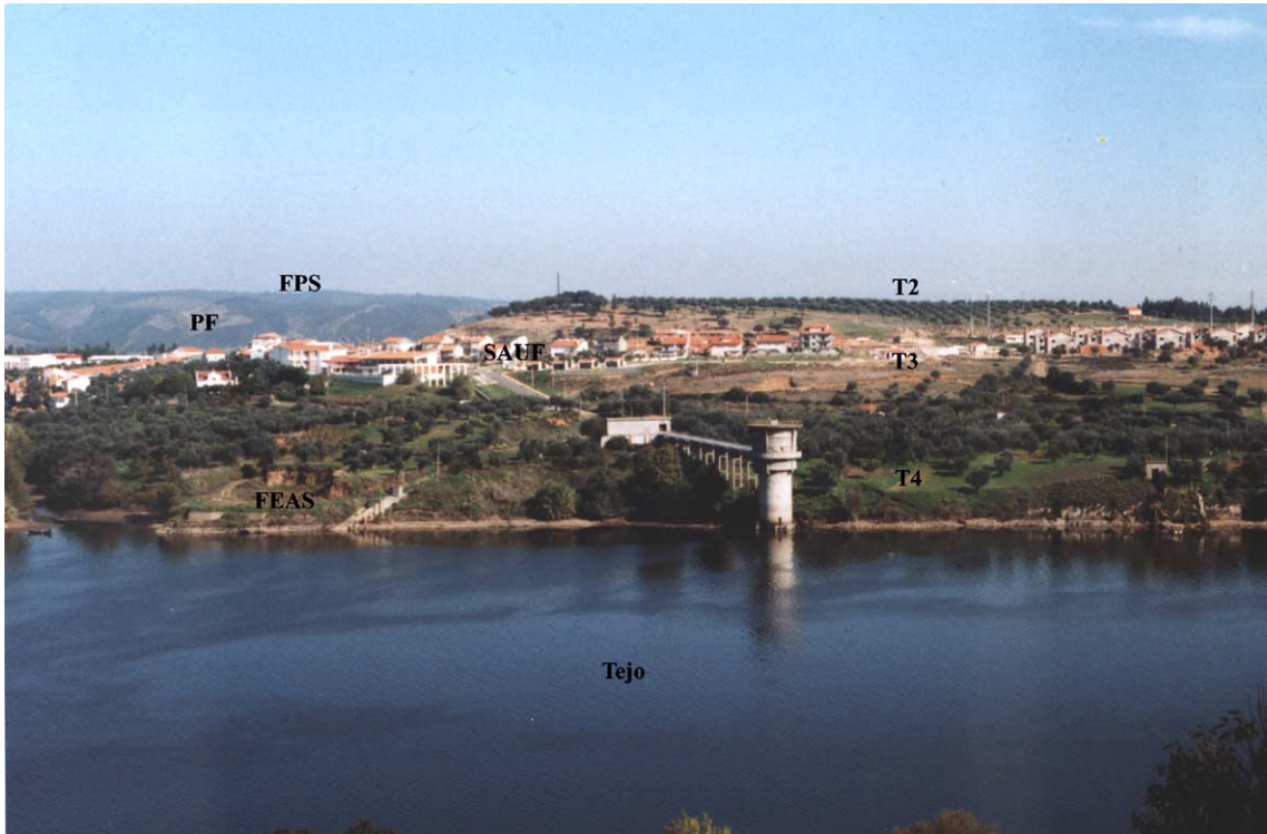
Fig. 13. Terraces at the Vila Velha de Ródão área. The terrace T2 (older) is tilted towards southeast (gradient: 3.4%). FPS—Fundamental planation surface; PF—Ponsul fault scarp; T2, T3 and T4—terraces; FEAS—Foz do Enxarrique archaeological site; SAUF—Senhora da Alagada urbanization fault (outcrop).
