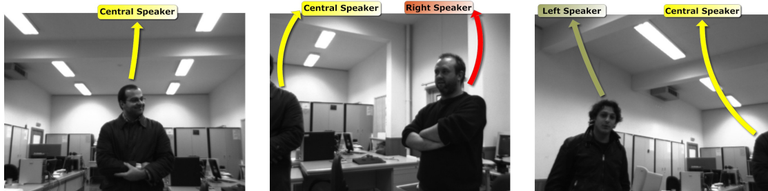
(a) Left camera snapshots corresponding to chronologically ordered time-instants. Three male speakers are maintaining a dialogue, at 18^\circ , -2^\circ and -35^\circ azimuth respectively relative to the Z axis, which defines the frontal heading respective to the IMPEP “neck”. As can be seen on the first frame, only the centre speaker is initially inside the stereovision region-of-interest for processing, being the remainder two speakers consecutively scanned as a result of active exploration-driven gaze-shifts.
