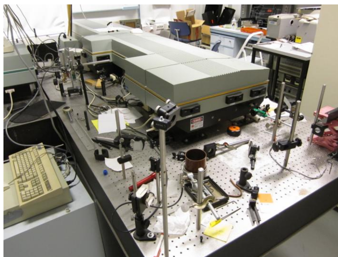
Figure 2.6 – OPO-based system (Continuum) providing 5-ns light pulses tunable in the 225 nm to 4 \mu\text{m} range (the pulse duration was \sim 5 ns, the spectral linewidth \sim 0.1 \text{cm}^{-1} and the repetition rate 10 Hz) used in the Laboratory of Physical Chemistry, Department of Chemistry (University of Helsinki).
