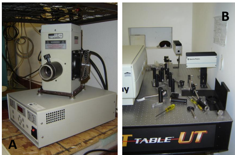
Figure 2.5 – Irradiation sources used in the Laboratory for Molecular Cryospectroscopy and Biospectroscopy (LMCB) – Coimbra: A: 500 W Hg(Xe) lamp (Newport, Oriel Instruments), B: Quanta-Ray MOPO-SL pulsed (10 ns) optical parametric oscillator (FWHM \sim 0.2 \text{cm}^{-1} , repetition rate 10 Hz, pulse energy E 1.0 mJ) pumped with a pulsed Nd:YAG laser.
