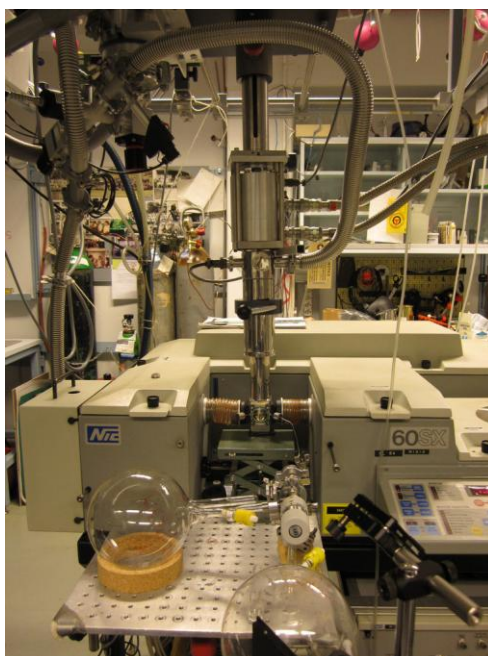
Figure 2.4 – Nicolet 60SX Fourier Transform infrared spectrometer at the Laboratory of Physical Chemistry (Department of Chemistry – University of Helsinki).
