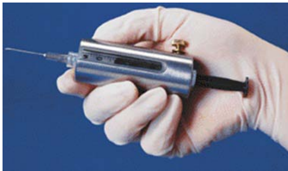
Figure 4.6 – Lead protection for a radiopharmaceutical's syringe. From [78].
