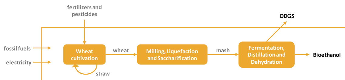
Fig. 4.4. Flow chart illustrating the bioethanol production chain from wheat. Transportation activities, potential blending with gasoline and combustion are not shown for the sake of simplicity.
