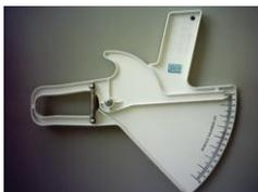
**Figura 11.** Adipómetro SLIM GUIDE® (P= 10g/mm<sup>2</sup>)
