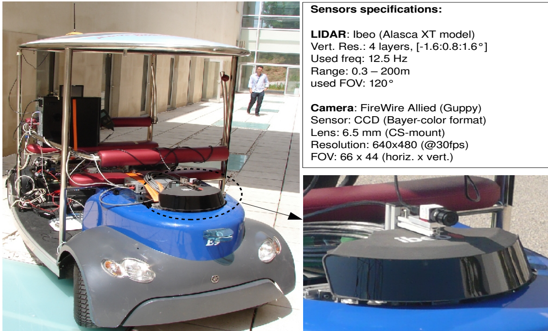
Figure 6.3: ISRobotCar: a electric vehicle and its sensors setup, enlarged at the bottom-right part, used in the dataset collection. A short specification of the sensors are presented at the top-right side of the figure.
