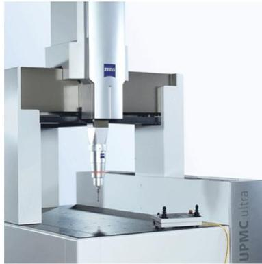
**Fig 3.5-1 - Coordinate Measuring Machine**
