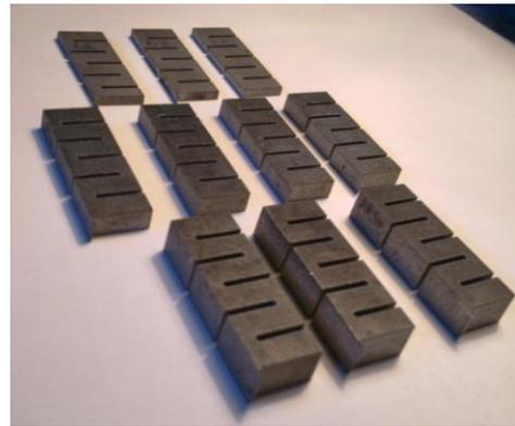
Fig 3.8-5 - All Comb workpiece (2 mm, 4 mm and 6 mm)
