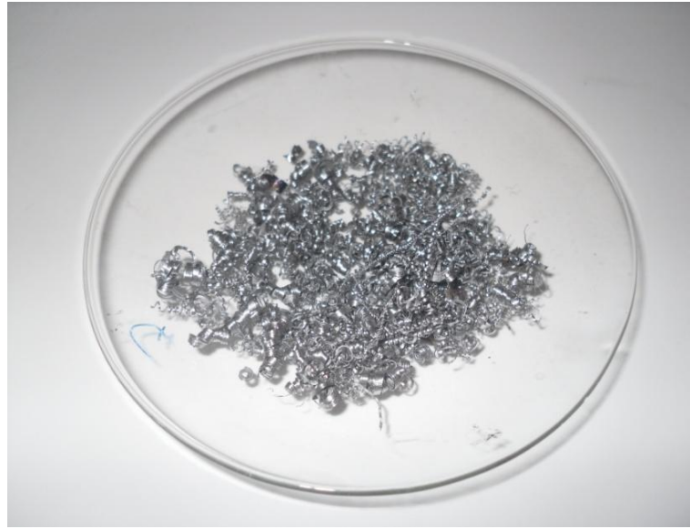
Fig. 5.12 - Iron shavings (from a metal turner) used in the laboratory experiments.
