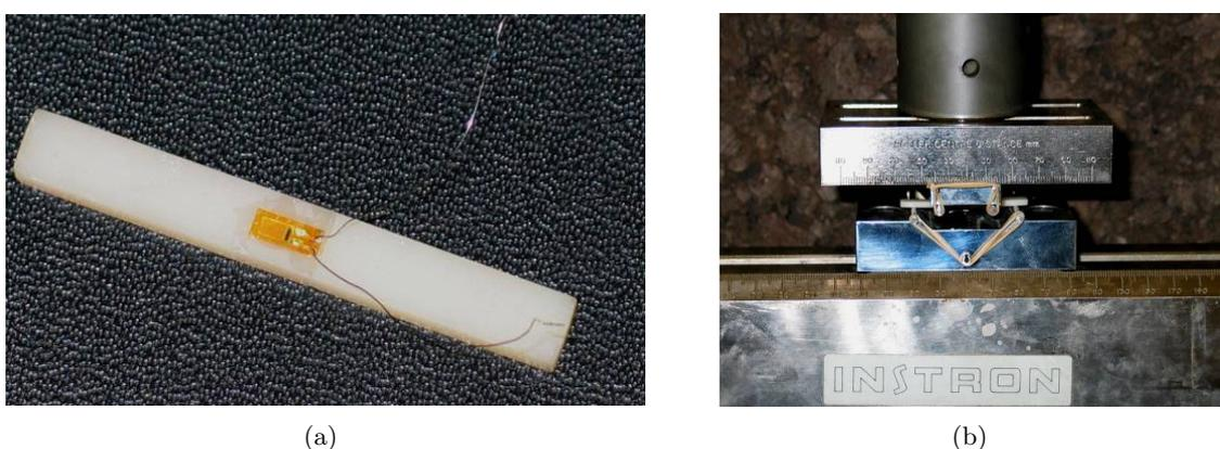
Fig. 3.5: a) Dental composite specimen's prismatic shape; b) Experimental assembly with specimens in place during test.
