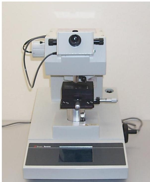
Fig. 3.4: Struers hardness testing equipment, model Duramin used to perform Vickers microhardness tests.
