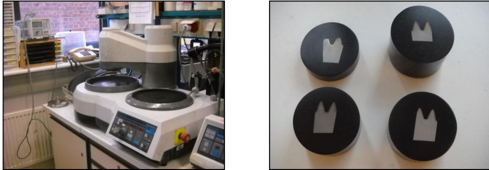
Figure 16 - Equipment used for sample polishing and samples after being processed in plastic.
