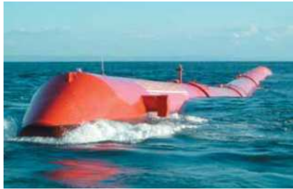
Figure 1. A Pelamis wave energy converter in the water (Pelamis Wave Power, 2011a)
