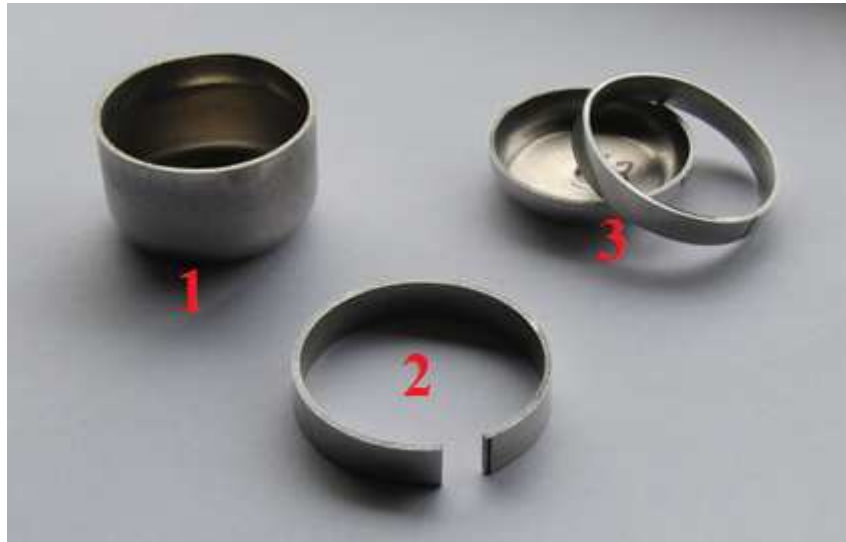
Figure 3 – Split- ring test, 1 – initial cup, 2 – split-ring, 3 – cup’s bottom and top after the trimming of the ring.
