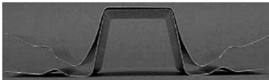
Figure 2 – Example of springback in a rail [Hsu et al, 2002].
