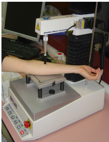
Figure 4.5 In vivo evaluation of the films bioadhesion to human skin using a TA.XTPlus Texture analyzer.
