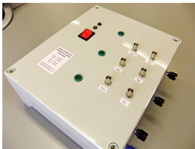
Figure B.13: Final module of the three-phase voltage and current measurement board.
