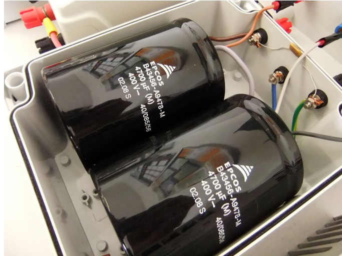
Figure B.3: DC bus capacitors power module with two Epcos 400 V 4700 \mu F capacitors.
